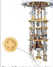
Figure 3 Quantum computer chips within a cryogenic environment. Image courtesy Rigetti Computing. Photo by Justin Fantl.
